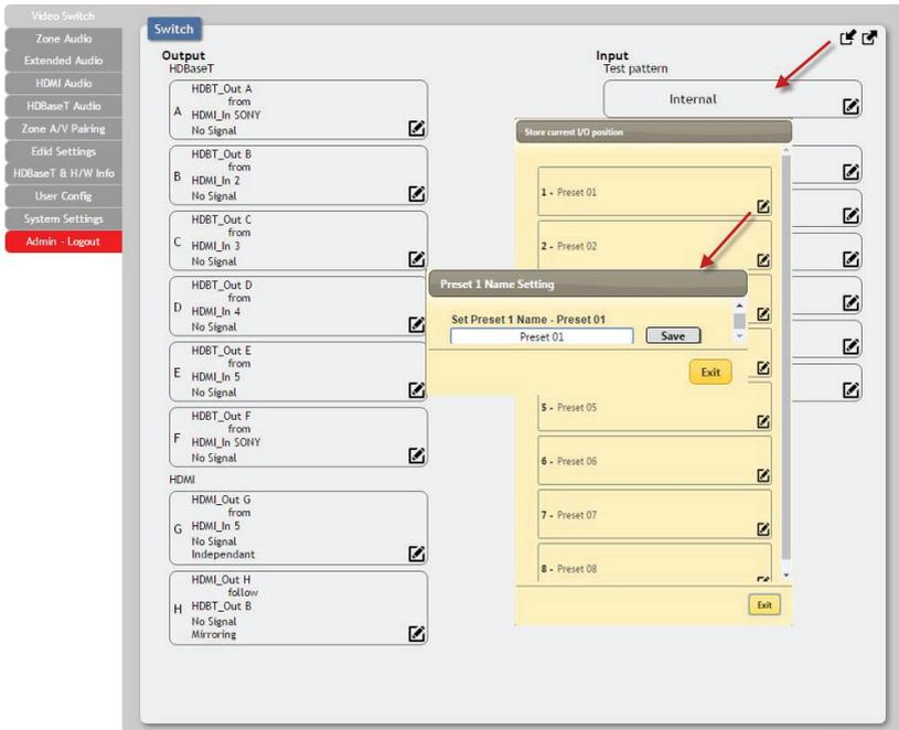
This matrix can store up to eight video and audio routing presets. Presets can be utilised to store multiple different routing states in advance for rapid, hassle-free, recall.
