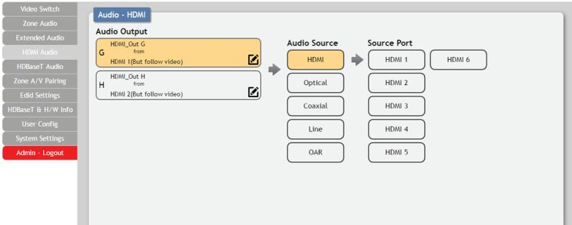
Click the buttons from left to right to choose each output's source. Once the new source has been selected, the change will happen immediately. Audio source options include HDMI, Optical, Coaxial, Line, and OAR.
