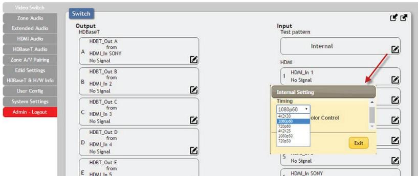
**Timing:** Test patterns can be generated with the following standard timings: 720p@50/60Hz, 1080p@50/60Hz, 4K@25/30Hz. Test pattern output does not use HDCP.
