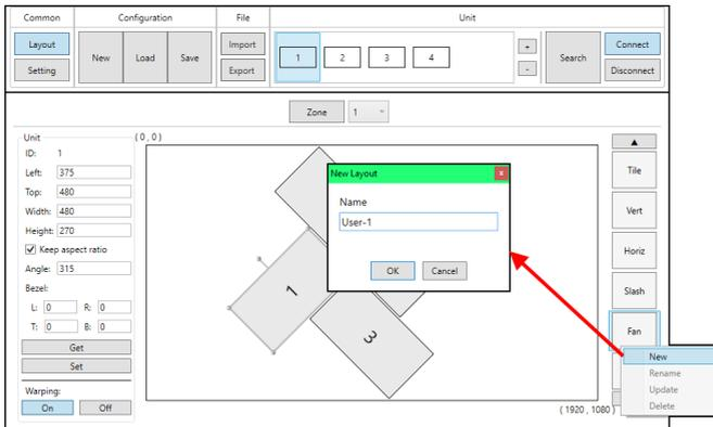
This control software provides a number of common, pre-defined, video wall configurations, however in most cases a customised layout will be needed. Custom layouts are created by selecting a layout to use as a basis, and then right-clicking on the layout’s selection button and selecting “New” from the dropdown. You then provide a name for the new layout and click “OK” to generate it. Custom layouts are coloured differently to make them easy to identify.
