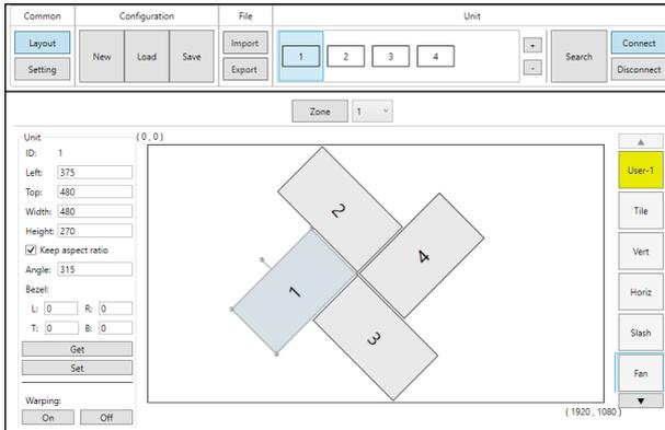
In addition to video wall design, creation, and positioning, this software can also be used to configure the scaler mode of the unit, if needed.
