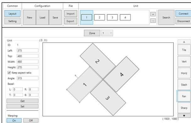
This control software provides a number of common, pre-defined, video wall configurations which can be selected and easily applied to any connected units. All pre-defined configurations are designed around video walls containing 4 displays.
