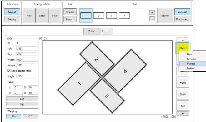
**1) Unit Information and Details:** This section displays all of the relevant position, dimension, and orientation details of the selected unit/display.
