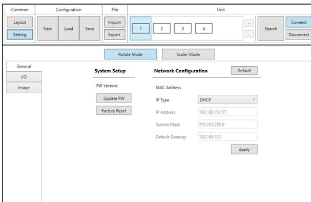
1) **System Setup:** Displays the current firmware version and provides options to update the firmware or perform a factory reset on the unit.
