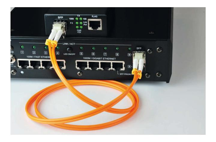
much noise and jitter its systems can remove. There are several advantages to a media converter such as the MC01, including galvanic isolation (which always reduces noise) and the fact that it reconstructs the signal at the receiver which reduces jitter.
