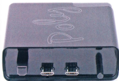
The Poly's connectors slide into Mojo's digital inputs to provide its streaming functions.
