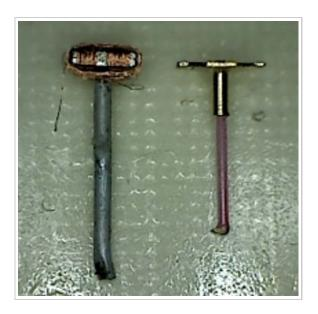
On the left is a Moving coil armature, the right is our tiny permeable flux modulator. You can see by the obvious size differences that the moving-coil system has greater mass, which means much higher inertia.
