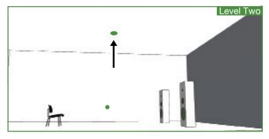
• Place (1) Dot on center of ceiling, halfway between speakers and listening position.
