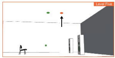
• Place (1) Dot within the center of ceiling, halfway between speakers and first Dot.
