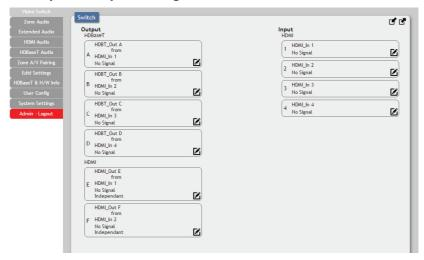
To begin assigning a new video route, please click the button of the HDBaseT output you wish to send video to (e.g. "HDBT\_Out A") and then click on the button of the preferred HDMI input port (e.g. "HDMI\_In 1"). If desired, you may select more than one output prior to selecting the input. As you select each button they will change their colour to orange. The new route will become active immediately and the routing information displayed on the buttons will change accordingly.
