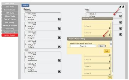
This matrix can store up to eight video and audio routing presets. Presets can be utilised to store multiple different routing states in advance for rapid, hassle-free, recall.
