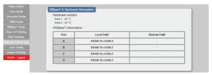
This page provides information concerning the temperature inside the matrix (areas 1 & 2) and the HDBaseT firmware versions used in the matrix and in connected receivers.
